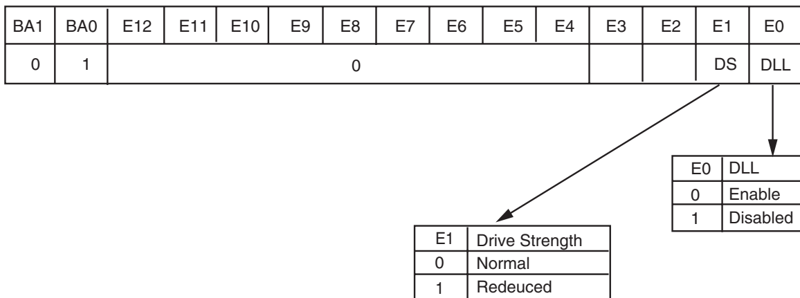
Figure 2: Extended Mode Register for DDR400
