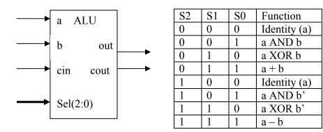
When S2 is high, the input **b** is inverted. This allows the FA to perform two's complement subtraction. Thus, when S = b"111", the **cin** input to the FA should be set to 1 (thereby performing b' + 1), i.e., subtraction.
