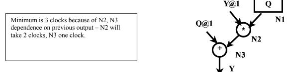
(5 pts) For the flow graph show below, if I pipeline the multiplier by one stage, what is the MINIMUM achievable initiation period (in clock cycles). A smaller initiation period means a faster initiation rate.
