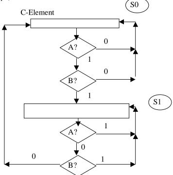
Assume the implementation uses one D-FF, and the state encoding is S0=0, S1=1. Complete the state table below, and draw the implementation of this digital system (show the DFF plus combinational gates that implement the ASM chart. Use an asychronous reset in your design to reset to state S0.
