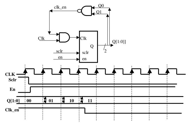
When  $clk_en = 0$ , clk signal to counter = 0, so counter does not count.
